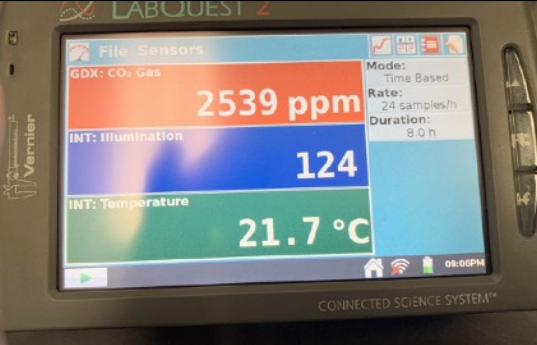
LabQuest set up to collect CO 2 data (below)
